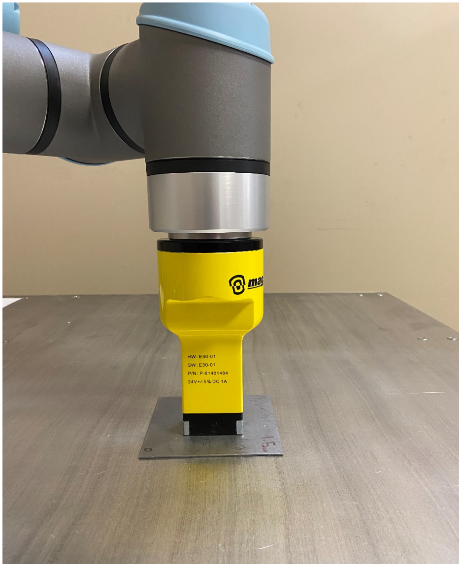
Fig 16: Example of Limiting Position 1 for Calibrated Part Present Signal
