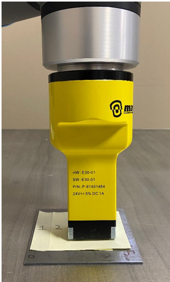
Fig 19: Example of Limiting Position 2 for Calibrated Part Present Signal
